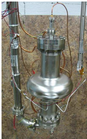
Drawing of single-cell \beta_g = 0.81 cavity and photograph of fine grain cavity on insert
