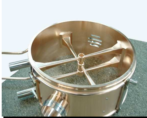
Resonator after brazing spokes and ports
