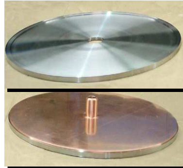
The double layer end-walls
