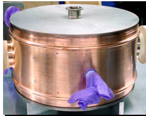
Resonator after welding of end-walls
