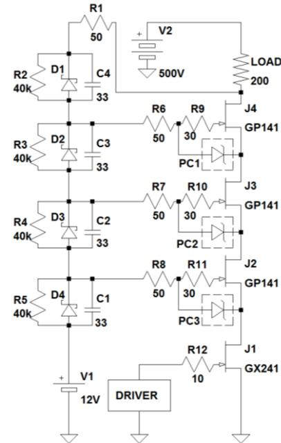
Fig. 3 – Simplified cascode switch circuit
