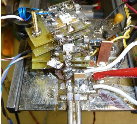
Fig. 6 – Cascode switch construction
