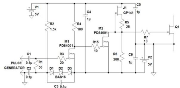
Fig. 5 – Drive stage circuit
