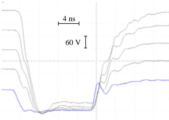
Fig. 7 – Drain voltages of all FETs
