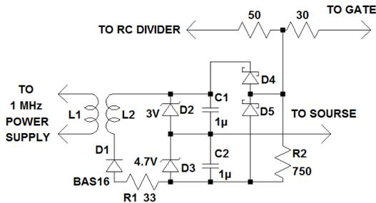
Fig. 4 – Voltage clamp circuit
